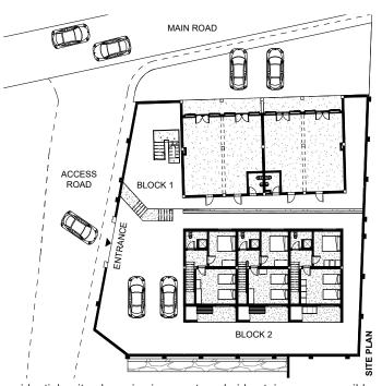
residential units above is via an external side staircase, accessible from a gated entrance off the side access road; Block 2 entrances are also accessed from this gate. The buildings are formed from reinforced concrete structural frames, infilled with Beehive's sitemade Hydraform blocks; these blocks are left un-rendered externally, to create attractive yet low-maintenance facades.
