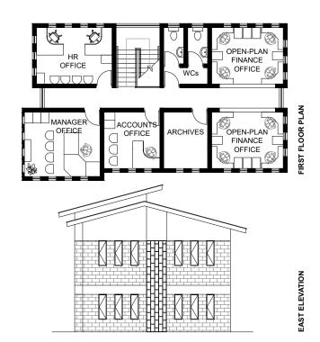
on-going maintenance costs are low. The rectangular windows are repeated around the building, and all are openable, allowing a good level of passive internal temperature control. The large open-plan office spaces have evenly-spaced windows along three facades, allowing decent levels of natural lighting throughout the year.
