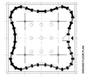
soil blocks, supported at regular intervals along the perimeter of the building by a series of blockwork piers, and the roof structure sits within the walls of the building, formed of four sculptural, tree-like timber columns. The columns are 'lifted' off the floor by steel feet, creating a light, filigree feel to the chapel's interior.
